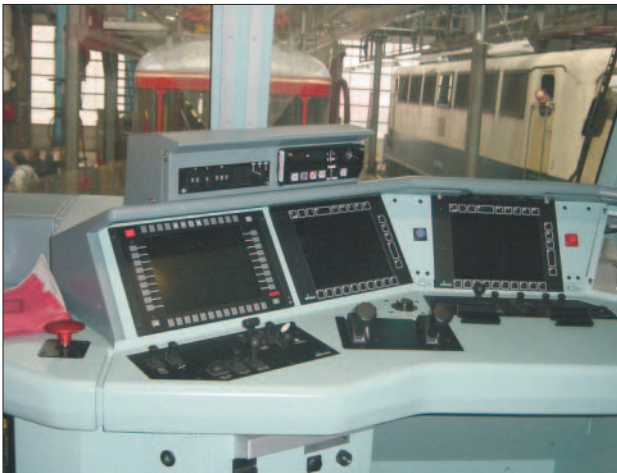
Fig. 5: The class 185's driver's console for hauling trains between Germany and France. Given the lack of interface uniformity, the operating elements for the French train-protection system have had to be placed on top of the regular monitors
