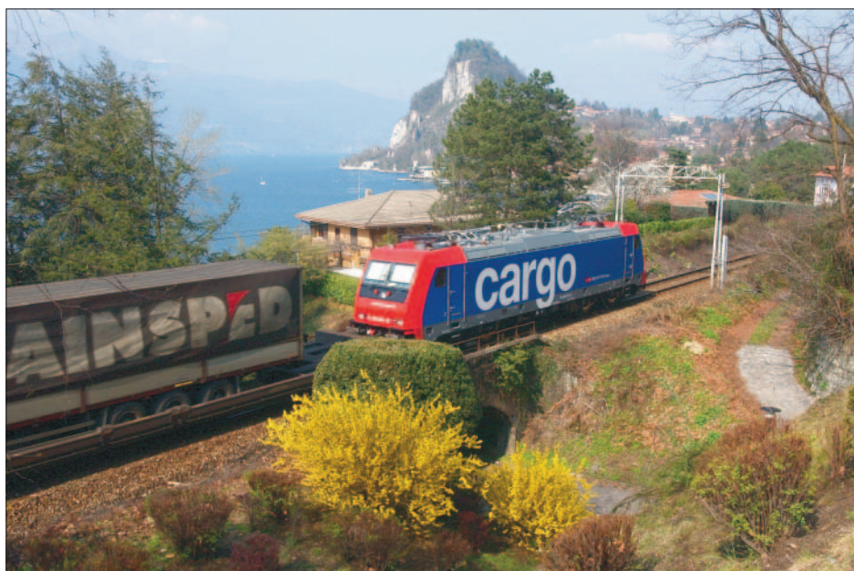
Fig. 7: An SBB/CFF/FFS Cargo class-“Re 484” locomotive hauling a shuttle freight train between Switzerland and Italy
